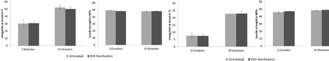
Figure 1b: EtO mechanical properties of EOS PA1101
